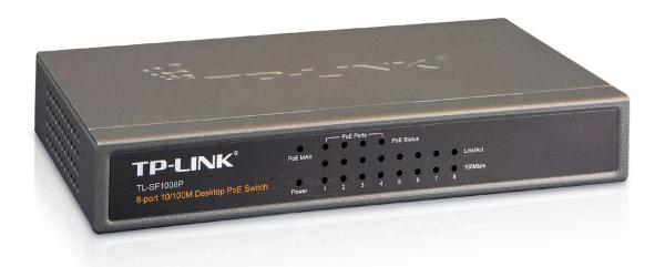
With four PoE ports, transfers data and power on one single cable Working with IEEE 802.3af compliant PDs, expands home and office network
