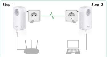
**Note:** Powerline adapters should be deployed on the same circuit and in set of two or more. The first, connected to the router and others located elsewhere to enable connectivity in those locations.
