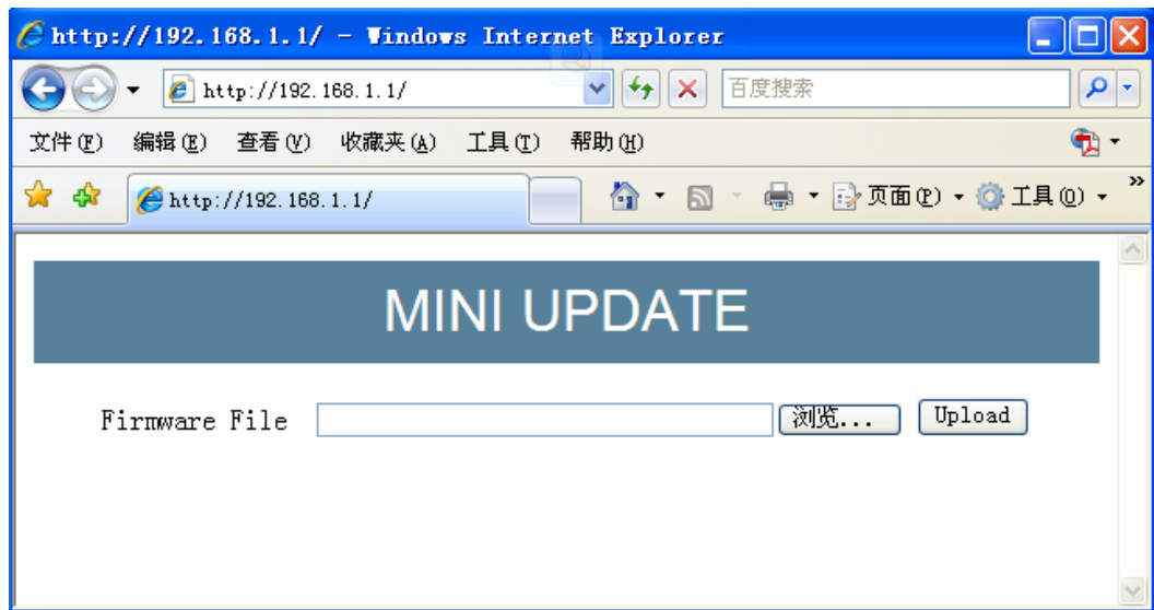
Figure 5-77 CFE mode upgrading
